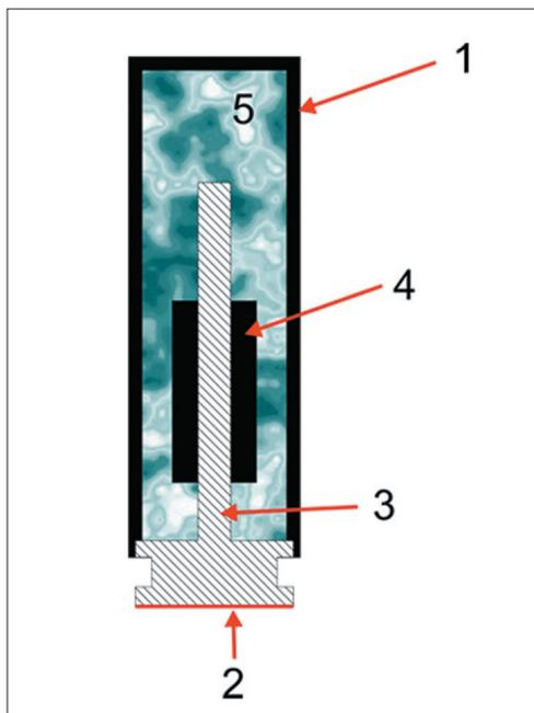
**Fig. 2.** Cold test applicator design (1 – polymer cylindrical body; 2 – working surface of the applicator (12.5 mm aluminum plate); 3 – aluminum core; 4 – silver coupling mounted on the aluminum core; 5 – working medium (2 ml deionized water))
